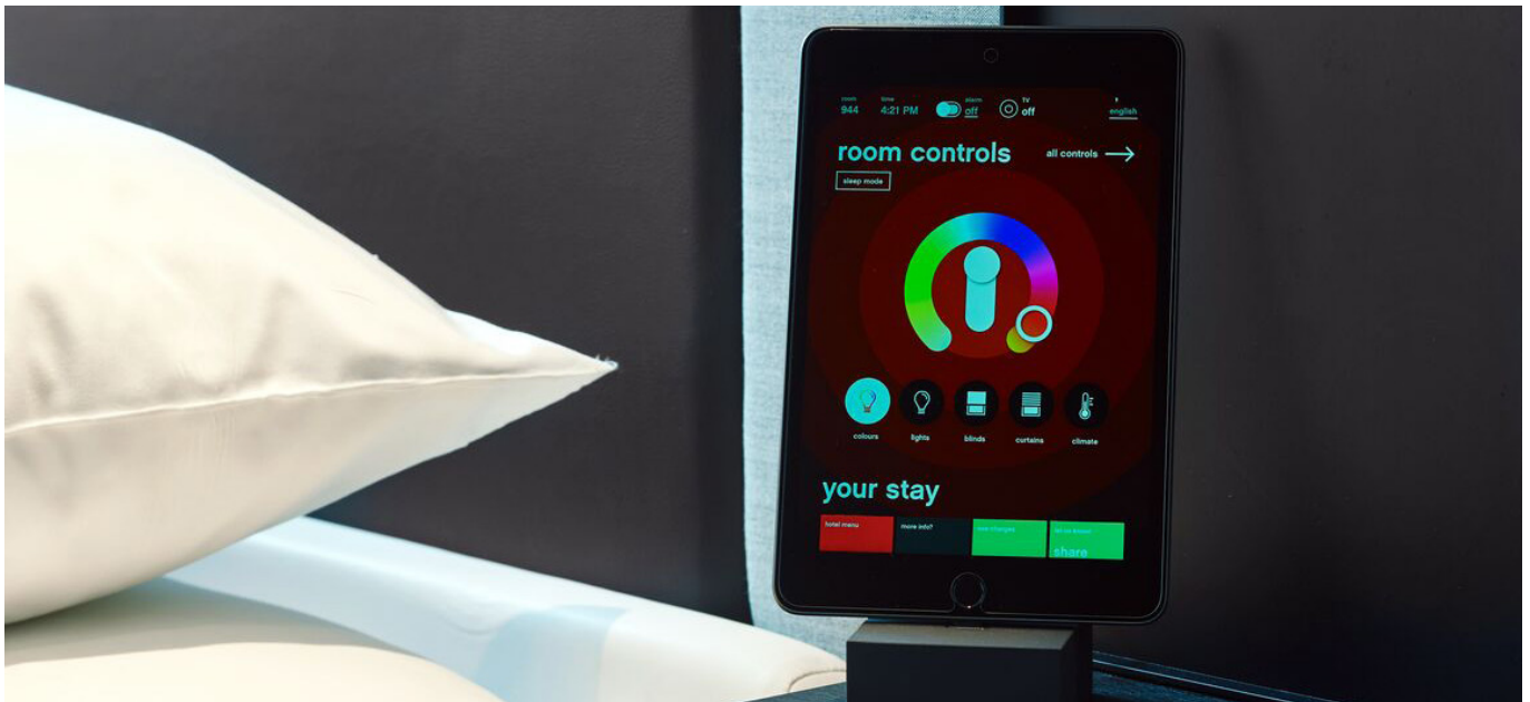
Figure 4 - Lighting controls via in room iPad.
